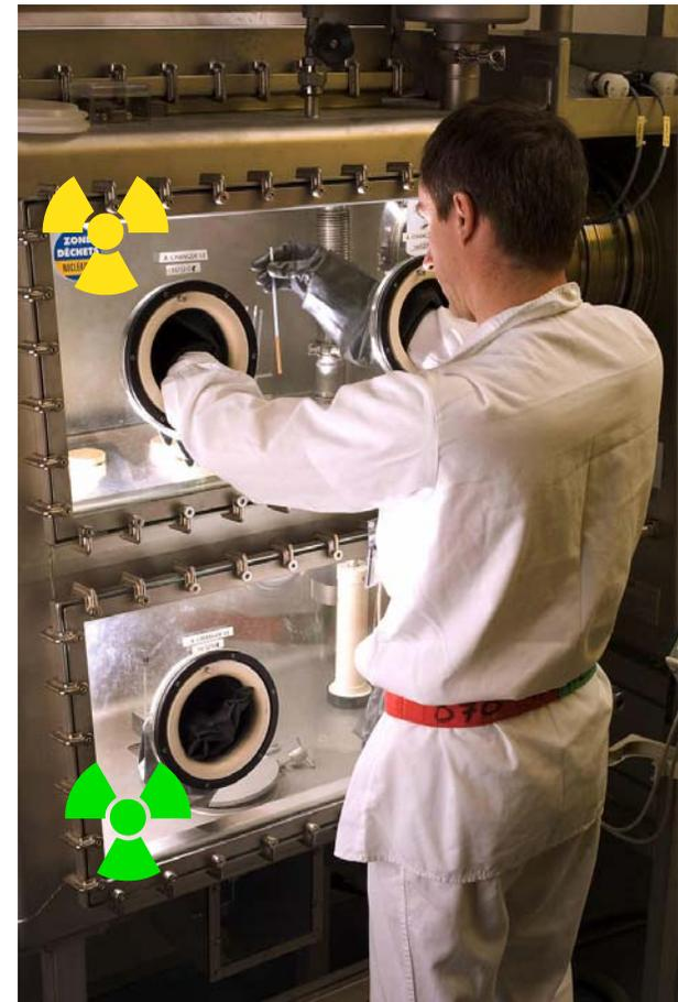
Safe and reliable management of radioactive liquid samples in use in Atalante lab.
