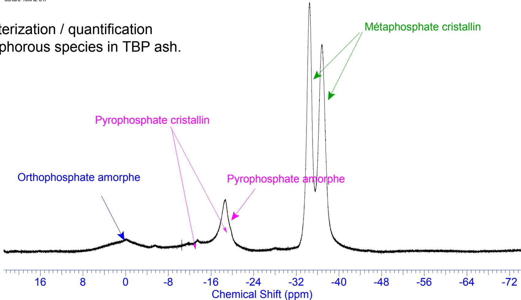
$^{31}\text{P}$  MAS spectrum about inactive ash 5mm probe 10kHz
