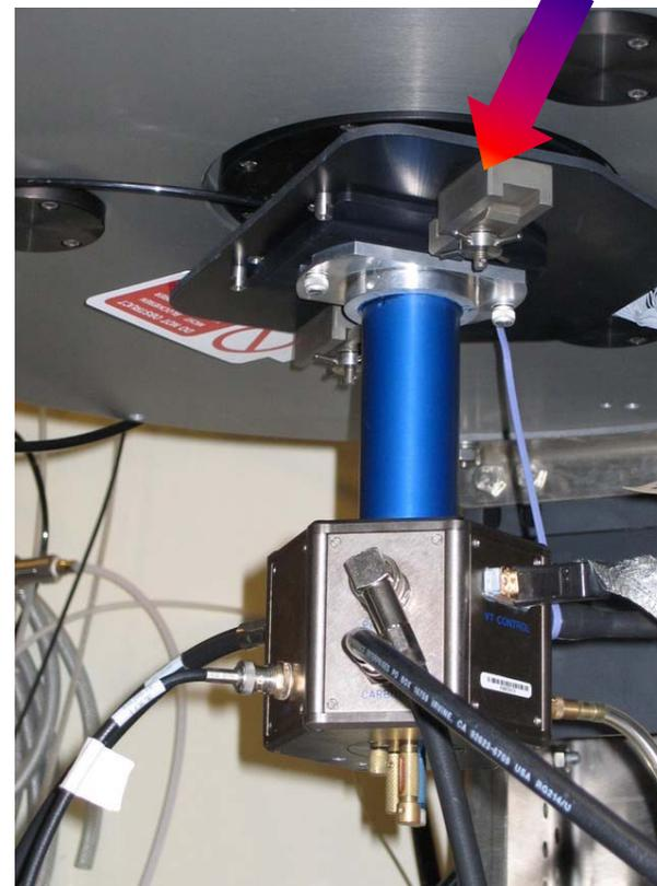
5mm Varian probe in a Varian narrow bore + adaptation for Bruker probes.
