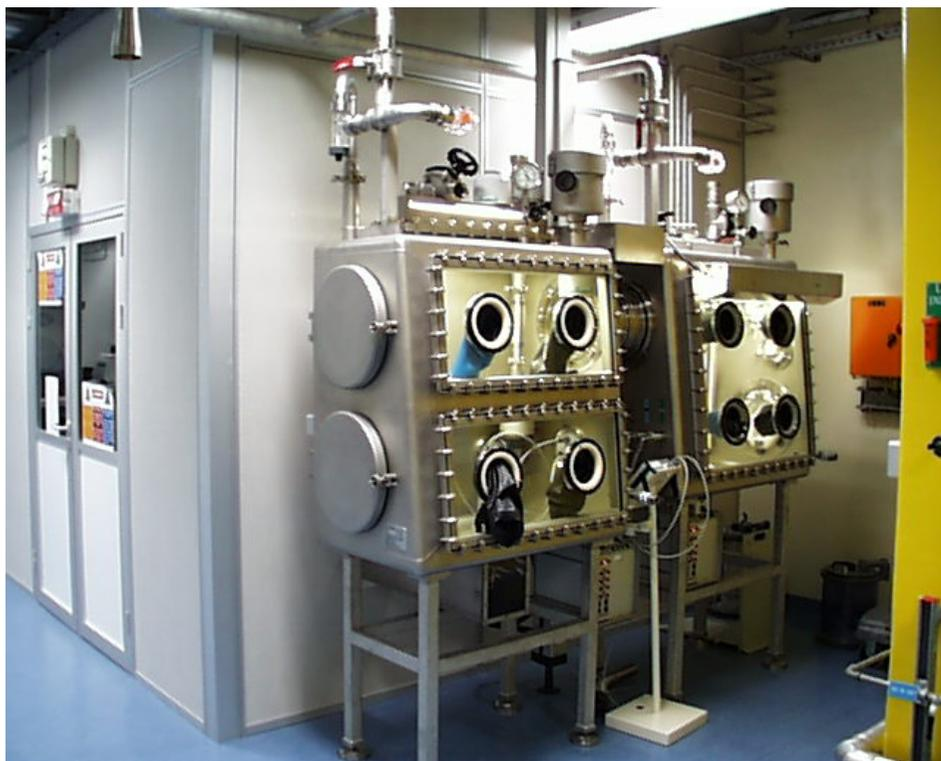
The two level glove box is linked to a normal glove box for the teflon tube conditioning.
