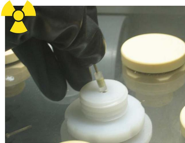
Commercial insert manage through a screw (drilled at the bottom)
