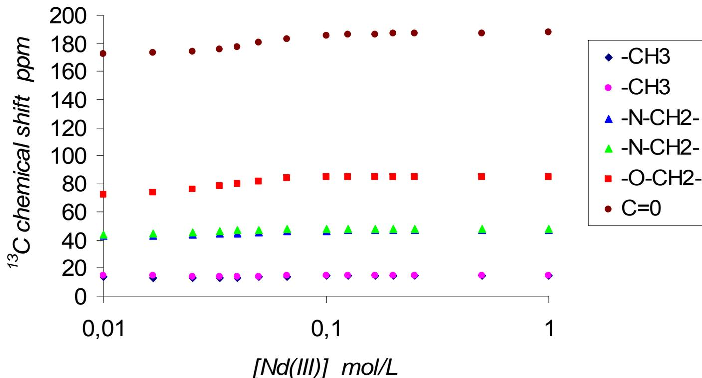
$^{13}\text{C}$  chemical shift vs  $[\text{Nd(III)}]$   $[\text{TEDGA}] = 0,1\text{M}$  at  $25^\circ\text{C}$  Ionic Strength:  $\text{NaNO}_3 = 1$ ;  $\text{pH} = 2$
